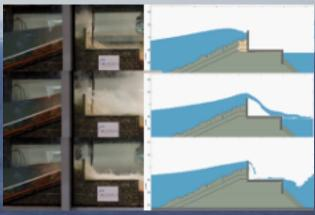
Comparison of the physical and numerical model experiments performed in ASTARTE (courtesy to UC) (top)
