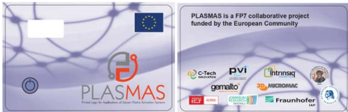
Figure 26 Smart card demonstrator within PLASMAS integrating an EC display and based on Cu circuits
