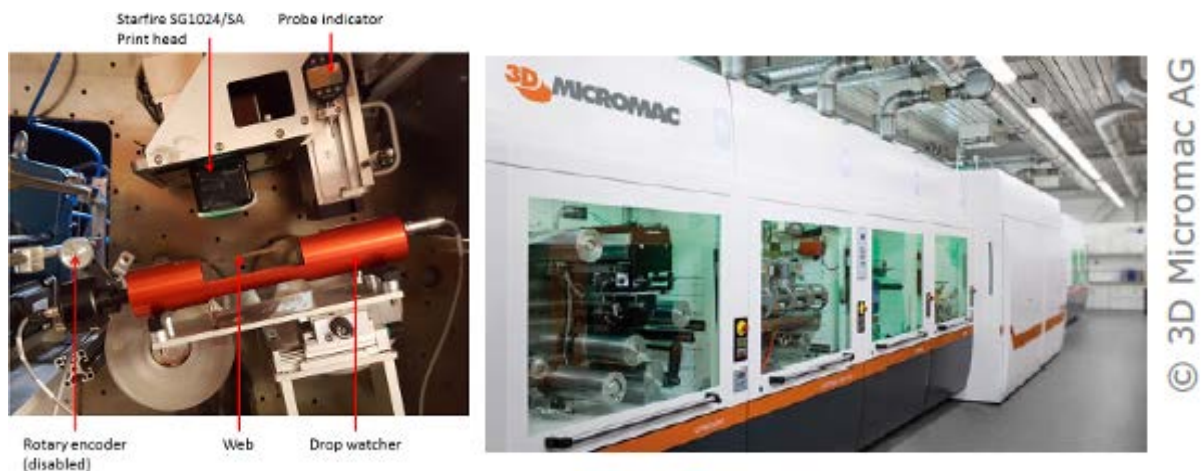
Figure 7 Industrial inkjet printer Starfire SG1024/SA and drop watcher installed in R2R machine (left) and Microflex R2R machine at 3DMM
