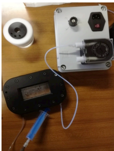
Figure 3.1.4. Picture and sketch of the flat recirculating miniphotoreactor for photoactivity testing in the liquid-solid regime. The photocatalyst can be in suspension or as a film deposited on the bottom window.
