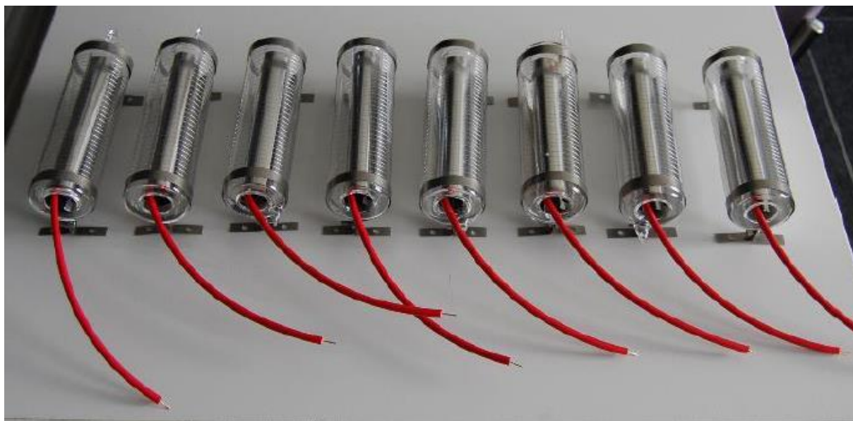
Figure 2: Excimer lamps units for Ovoshine prototype
