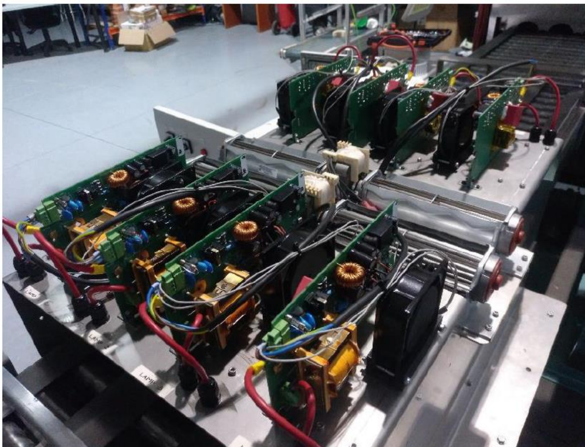
Figure 3: Power supply for Ovoshine prototype
