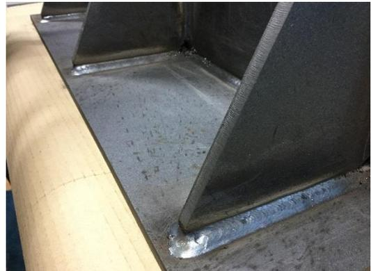
Typically, coatings thicker than 25-50 microns are necessary to achieve good protection against corrosion but this can lead to difficulties in the welding process due to the inability to strike a weld through the thick primer. Additionally, the incorporation of organic materials from the coating in the weld or entrapment of zinc fumes and gas can make the weld porous and have a significant negative impact on weld quality.
