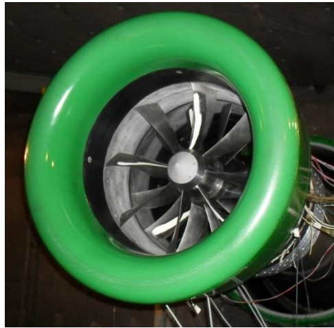
Figure 13: COBRA-Variant1 fan model installed at the C-3A test bench in CIAM.
