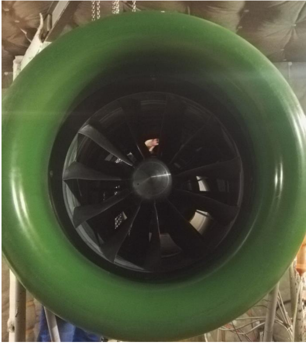
Figure 20: Mounted CRTF European variant on CIAM C-3A test rig.
