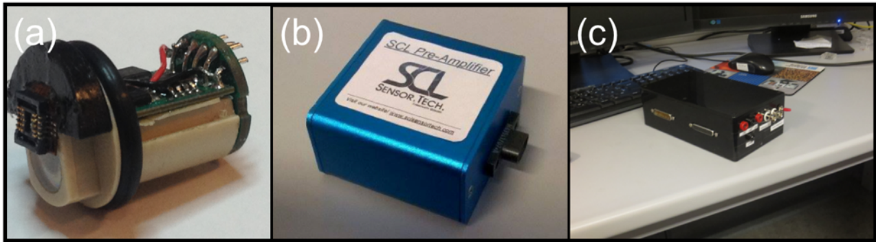
Figure 17: Key components for the FALCON upgrade module: (a) Newly designed AFM scanner nose upgrade for a Keysight 5500 AFM. (b) Post-amplifier box for the FALCON upgrade module. (c) Final Switch box for the FALCON upgrade module.
