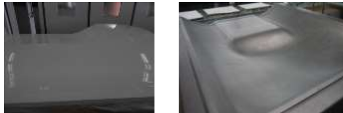
Figure 10. Manufactured master tool and final CFRP tool
