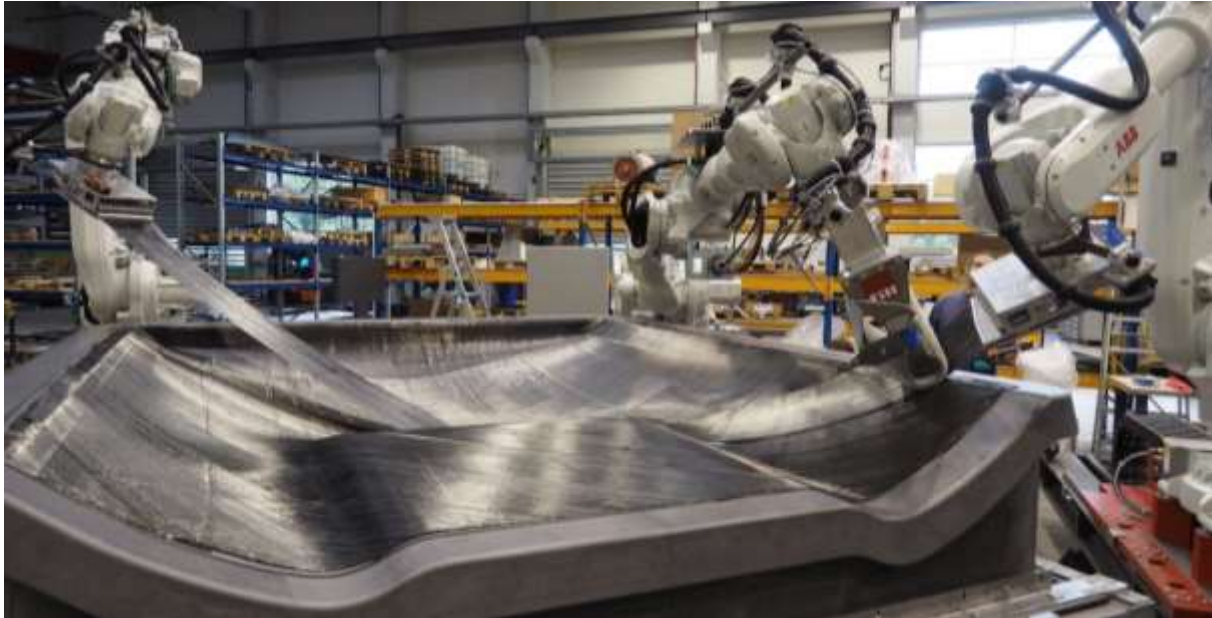
Figure 33. Full-scale tapelaying production cell running on test part production (truck front wall)
