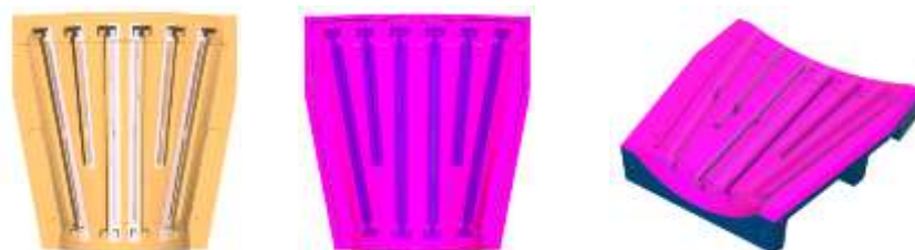
Figure 11. Preform tool, with membrane and inserts and the transferred membrane at the curing tool
