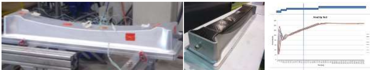
Figure 8. Final tool (heating test and with part) and heating ramp
