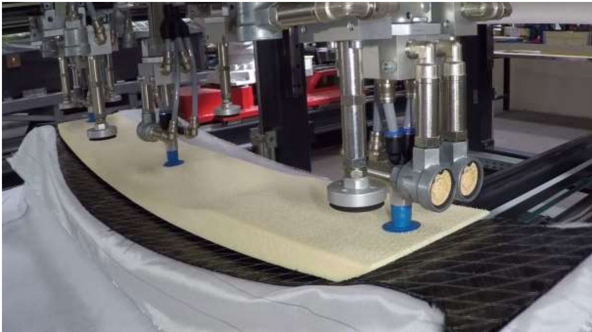
Figure 34. Automated positioning of the sandwich foam core for the automotive demonstrator.
