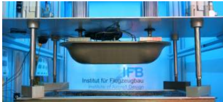
Figure 19. Mesoscopic simulation model of the draping process (top) and experimental draping test rig
