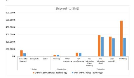
The next SME shipyard assessed have Fishing boats as their main product in their portfolio. The main effects of cost reduction when applying the SMART technologies occur in the Production phase, especially in the dock assembly process. The SMART technologies while implemented together in the shipyard can be de-
