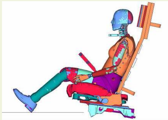
EvaRID (Eva female, RID – Rear Impact Dummy), world's first virtual crash test dummy representing average female
