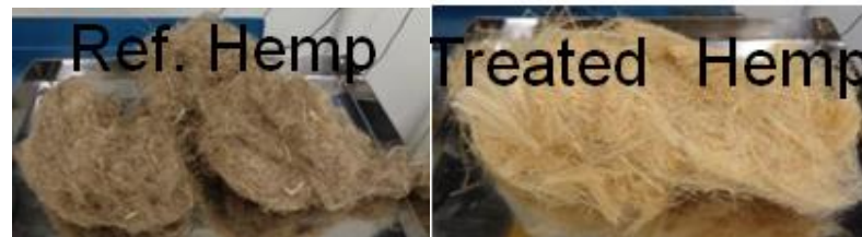
Figure 3. Left: Reference untreated hemp. Right: NATURTRUCK treated hemp fibre.
