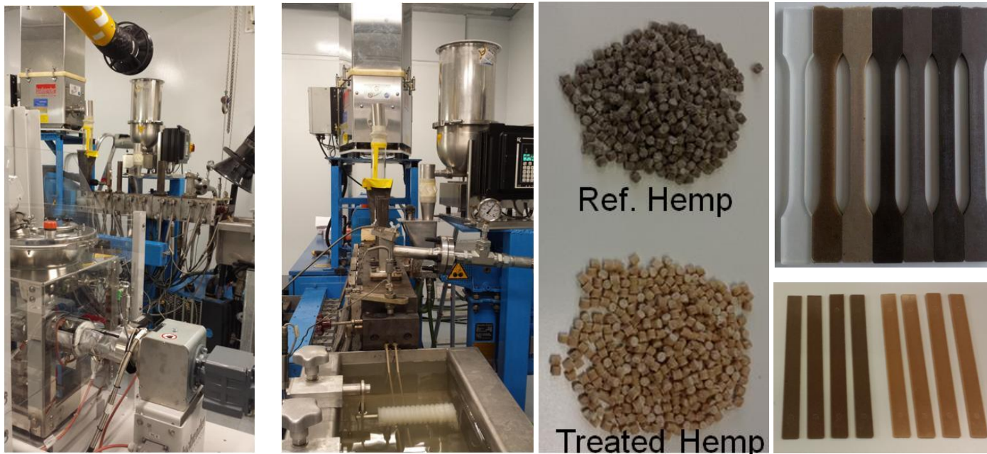
Figure 4. Left: COPERION ZSK25 TSE during the scale-up of NATURTRUCK compound. Center: NATRUCTRUCK compounds with reference and treated hemp fibres. Right: injected tensile and UL94 test specimens obtained from NATURTRUCK biocomposites.
