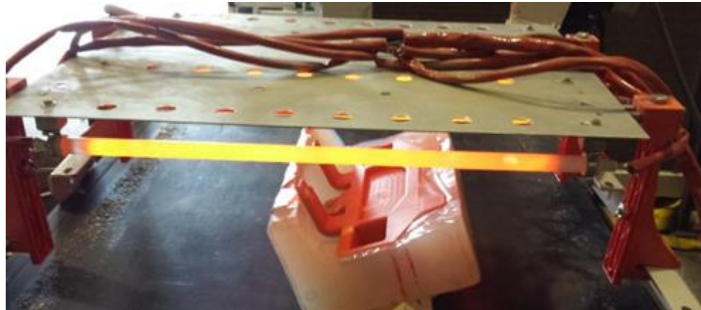
Figure 61. Continuous annealing of “bracket” part with IR using PLA biocomposite with threaded hemp fibres.
