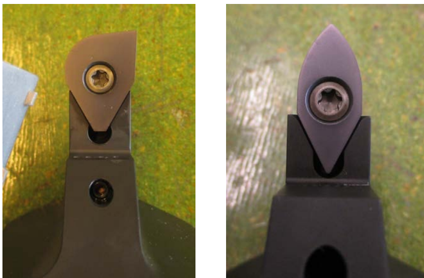
Figure 2.3.2: Novel hybrid tool insert prototypes
