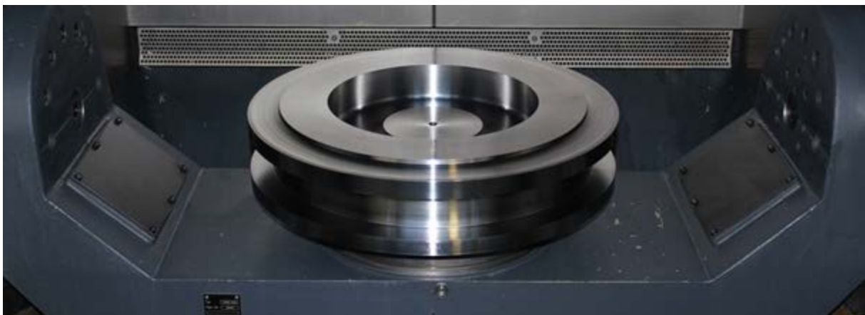
Figure 3.1: Demonstrator which was manufactured by simultaneous three axis turning / flexiSTAT technology.
