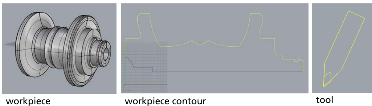
Figure 2.1.5: Use-case (workpiece and tool) to demonstrate the automatic tool path generation
