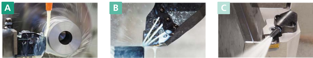
Figure 2.3.3: Different types of coolant supply. A: flood cooling (4bar), B: HP-cooling (70 bar), C: HP-cooling with injection nozzle (70 bar)
