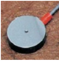
Figure 23: Load cell mounting
