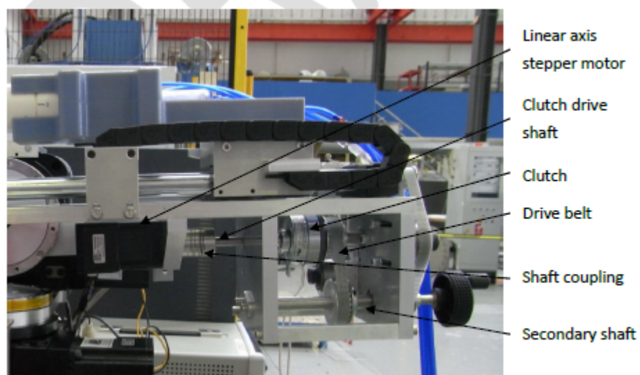
Figure 33. Clutch system description
