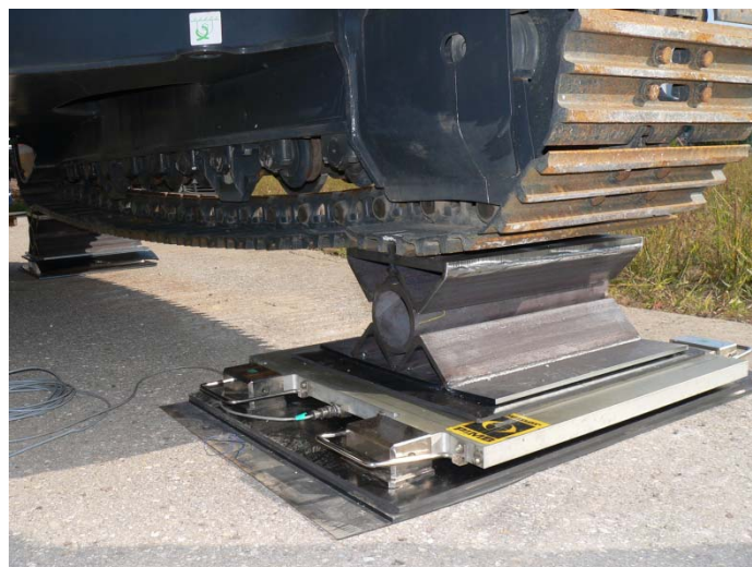
Fig. 5. View of one of the supports located at a measuring scale during measurements
