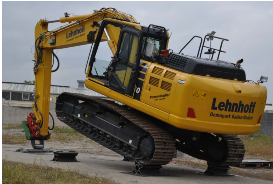
Fig. 6. Excavator setup on supports during determination of the vertical CoG coordinates
