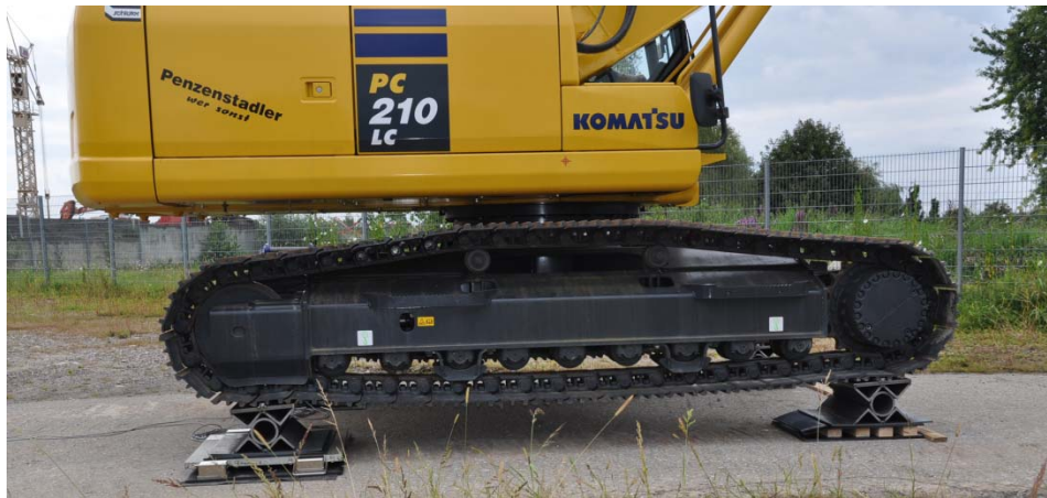
Fig. 4. Excavator setup on supports during the first series of measurements
