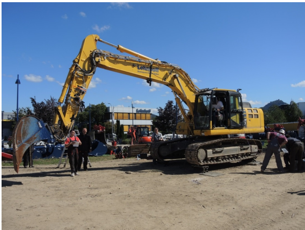
Fig. 12. Demonstrator installed on a Komatsu PC 210 excavator.
