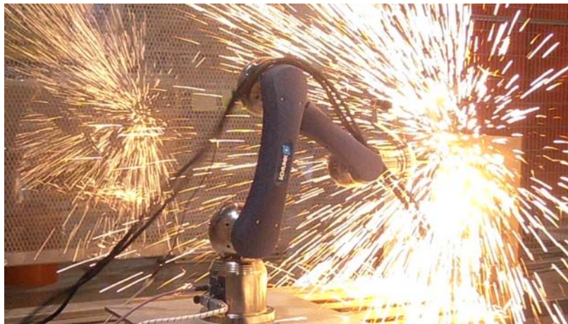
Figure 2 Welding trials using the manipulator
