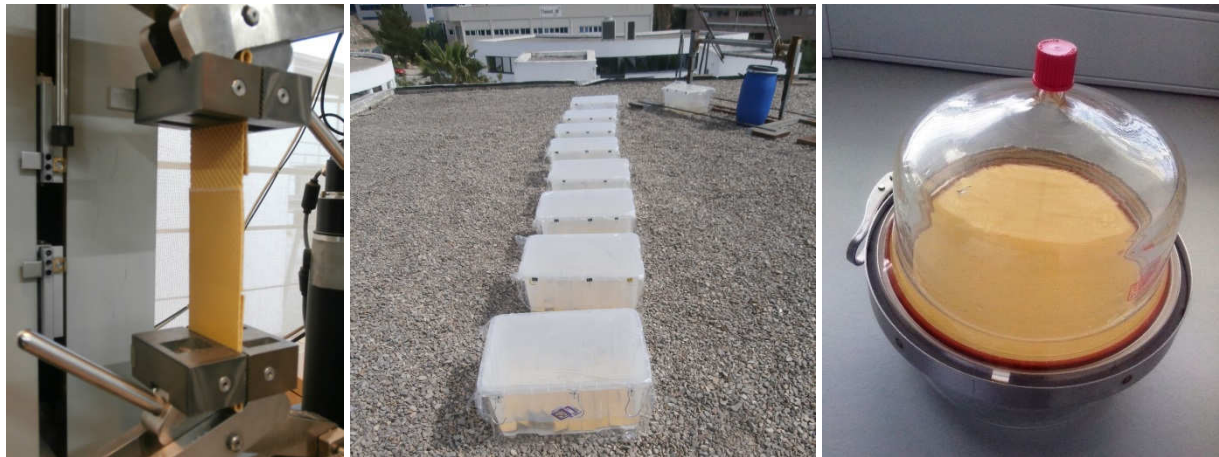
Figure 6. Welding resistance essay, aging test, sensory analysis at AIMPLAS
