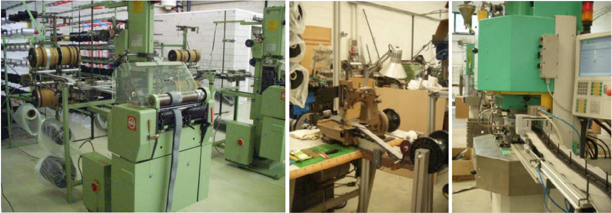
Figure 7: Loom weaving the tape, coupling of the cordon and overmoulding of teeth at ZIPLAST
