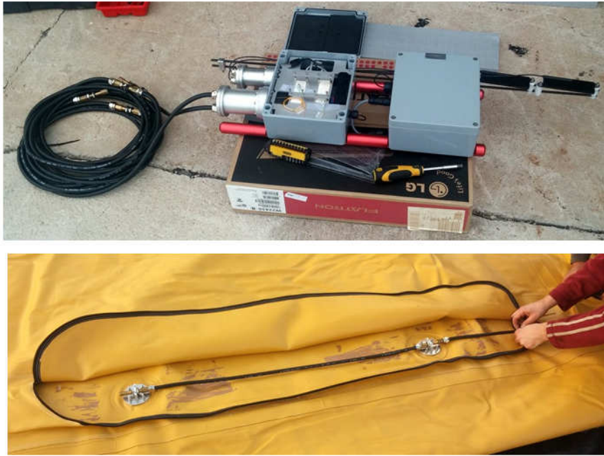
Figure 11: Fibre optics monitoring system during waterbag assembling.
