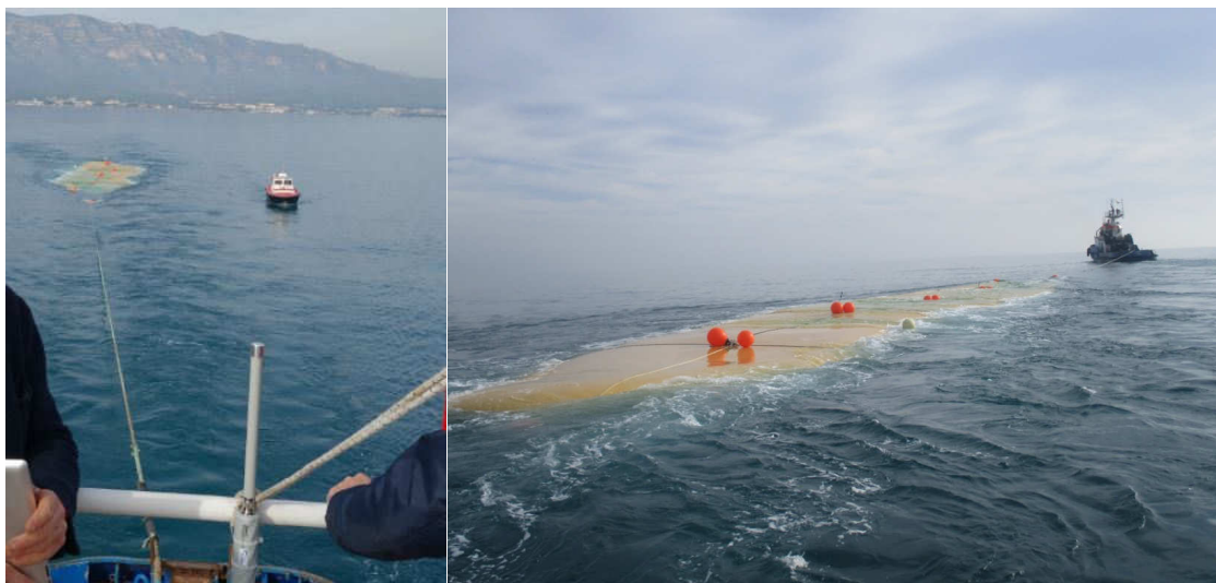
Figure 20: Waterbag in navigation seen from the tugboat (left) and support boat (right)
