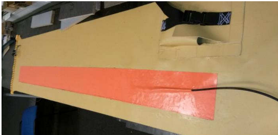
Figure 10: Sensor patch with glued fibre and attached fibre optic cable.
