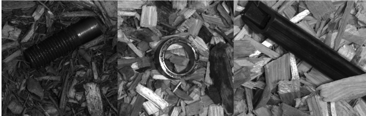
Figure 19 Sample images of the test objects and some of the fuel types used for training respectively testing the foreign object detection.
