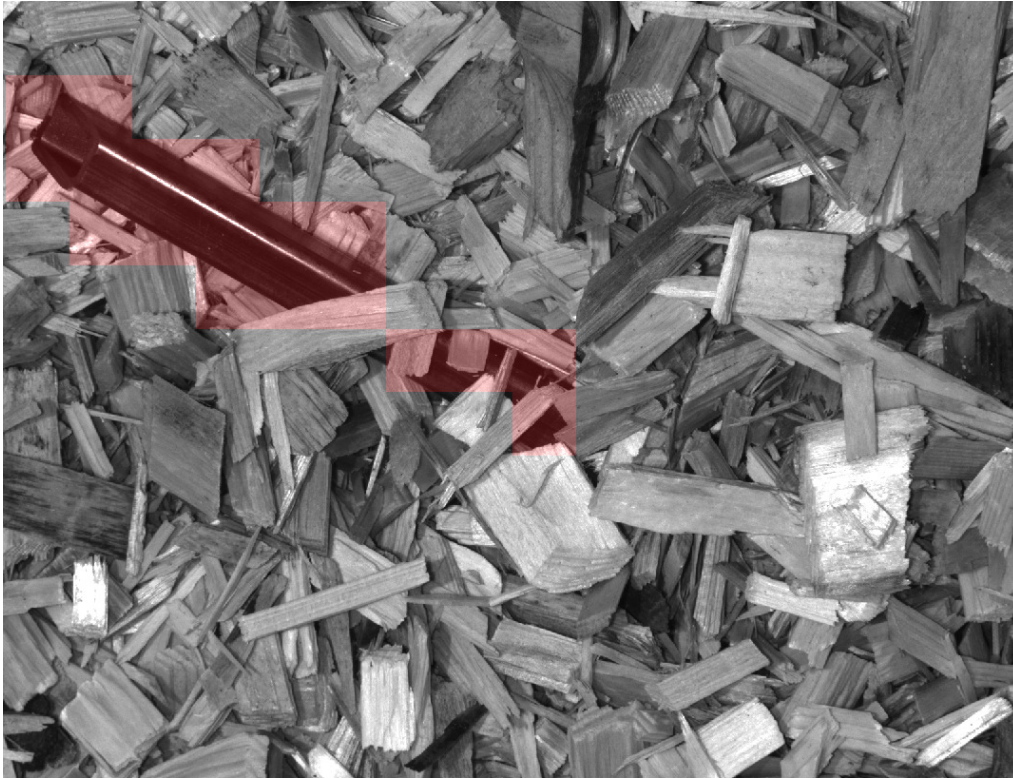
Figure 20 Example of a foreign object (steel strut) partially covered by wood chips. Patches detected by the system as foreign are marked in red.
