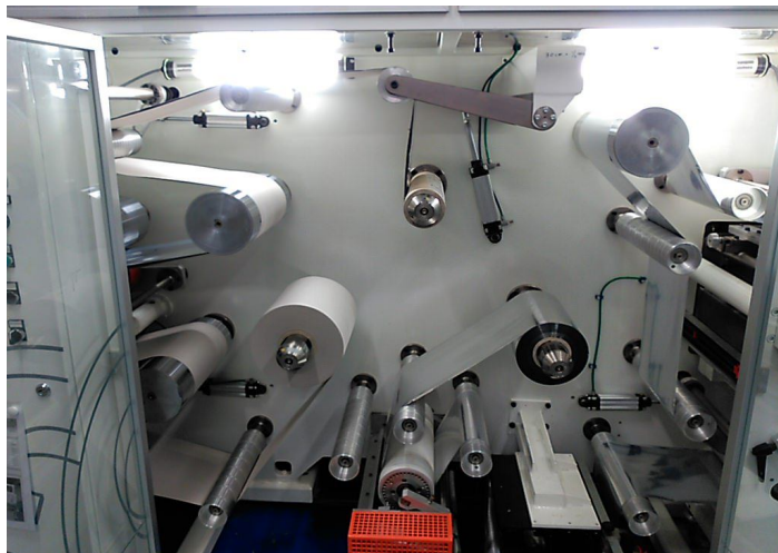
Figure 7. Pilot plant lamination set-up.
