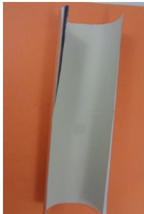
FIGURE 4. COATING / RECYCLED PAPER / METALLISED PET / PE COMPLEX PRODUCED (COATING SIDE) (CS2)
