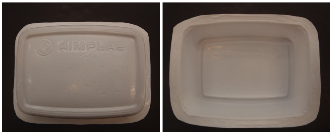
Figure 6. Example of thermoformed tray tested.
