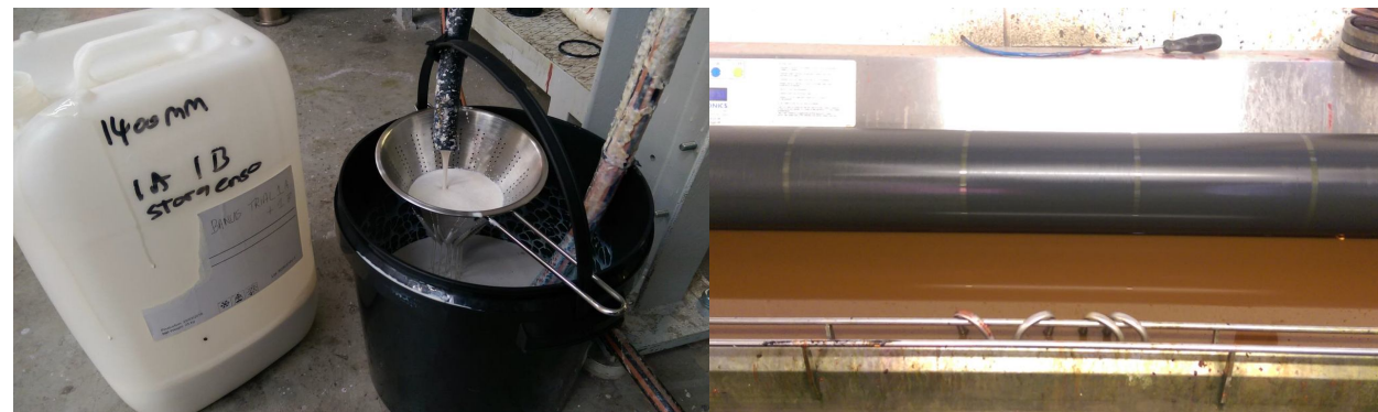
Figure 11. Left: Optimization of the coating viscosity. Right: Anilox coating rollers (CS3).
