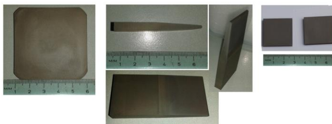
Figure 5: Bulk UHTC (ZrB 2 -WC-SiC) manufactured by Hot Pressing at CNR.
