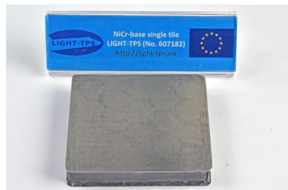
Figure 4: Overview of NiCr-base honeycomb panel prototype (single tile).
