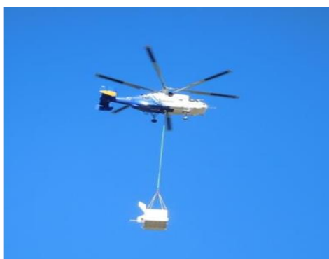
HyDrop on Kamov 32, 3 tons of Pellets, 500 ft. 60 Knots
