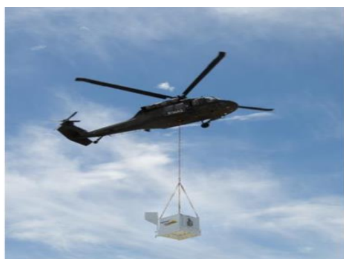
HyDrop on UH-60 Black Hawk , 2 tons of pellets 500ft., 60 Knots
