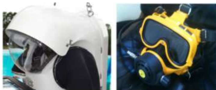
Figure 22: (Left) Helmet and visor mounting (Right) Used astronaut-diver's full face mask
