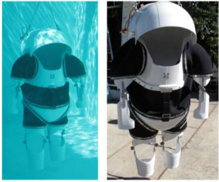
Figure 20: Prototype of the novel EVA training suit (Left) during first immersion at Comex (Right) Dry configuration before immersion
