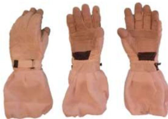
Figure 24: First iteration of novel training suit gloves
