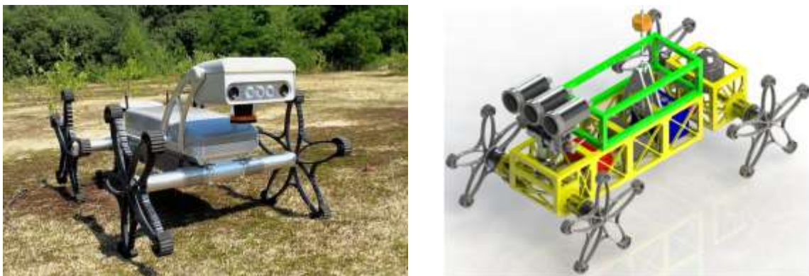
Figure 5: First robot design concept (right), based on ASGUARD legacy system (left)
