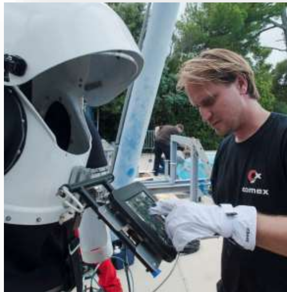
Figure 25: Tests of the gloves prototype in dry conditions on the HMI
