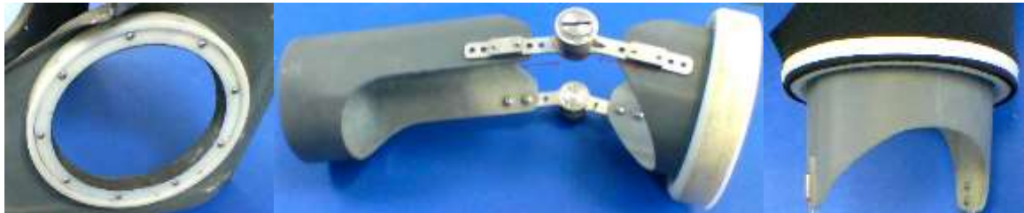
Figure 21: (Left) Shoulder ball bearing on the torso (Central) Torsion spring located on an elbow mounted on the arm assembly through adjustable tabs, the arm ball bearing is visible (Right) Neoprene soft part fixed on the arm ball bearing with clamp and screws
