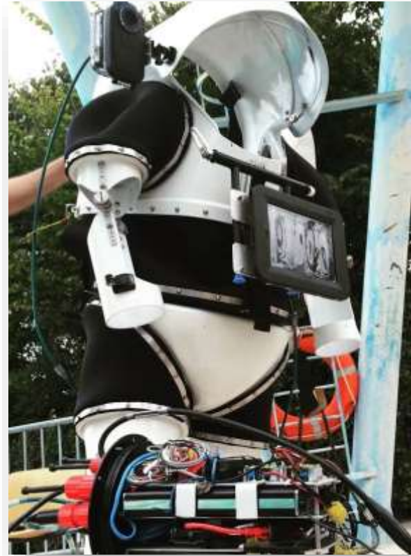
Figure 10 Spacesuit simulator with chest display in stowed configuration and Suit Computer Assembly (dismounted and opened) in the foreground.
