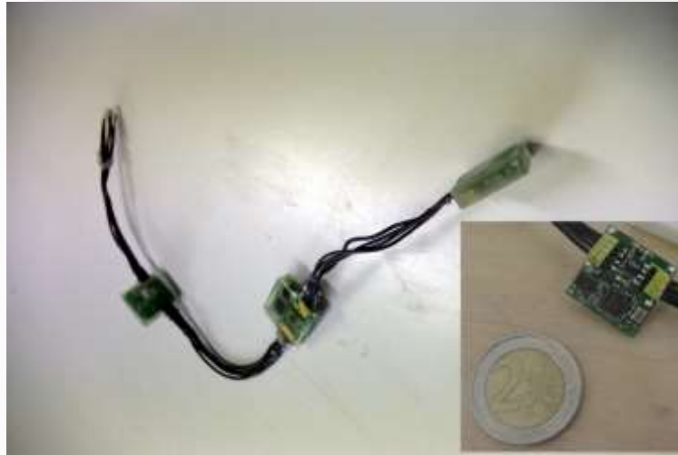
Figure 12 : Part of the sensor chain used to capture gestures. The depicted sensor string has been cast into epoxy for water-proofness. The smaller image shows the sensor's size.
