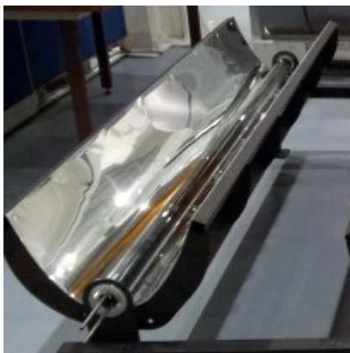
Figure 9. View of an individual CPC collector (left) and experimental efficiency curve of the collectors at 1000 W/m 2 (right).
