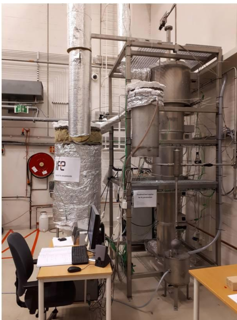
Figure 8 Fluidized bed for the proof-of-of concept of the SER reactor
