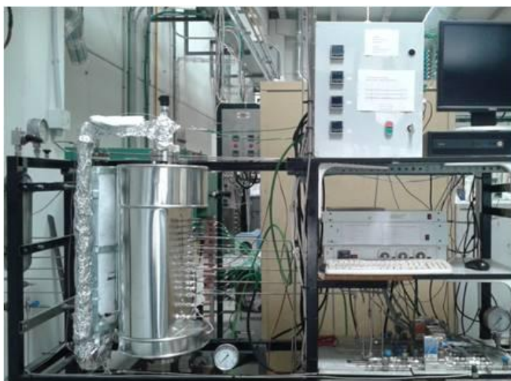
Figure 4 Experimental fixed bed reactor used at ICB-CSIC.
