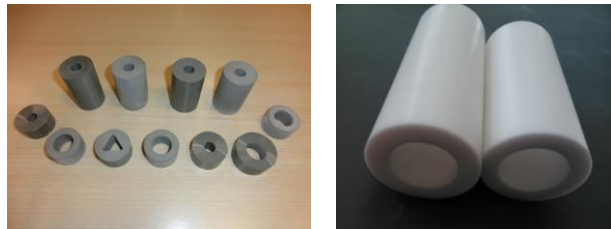
Figure 5: Example of the ceramic dies obtained for the prototypes production.
