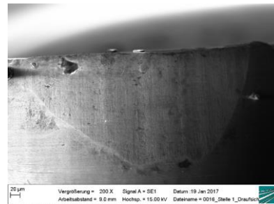
Figure16. SEM picture, edge of EFFIPRO tool after testing
