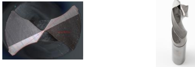
Figure 12: Prototype No 2: left: Drill head front picture. Right complete tool (brazed head to the shank)
