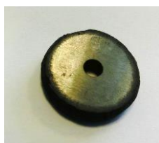
Figure10. Blank for prototype No 1 with edm'ed internal hole.
