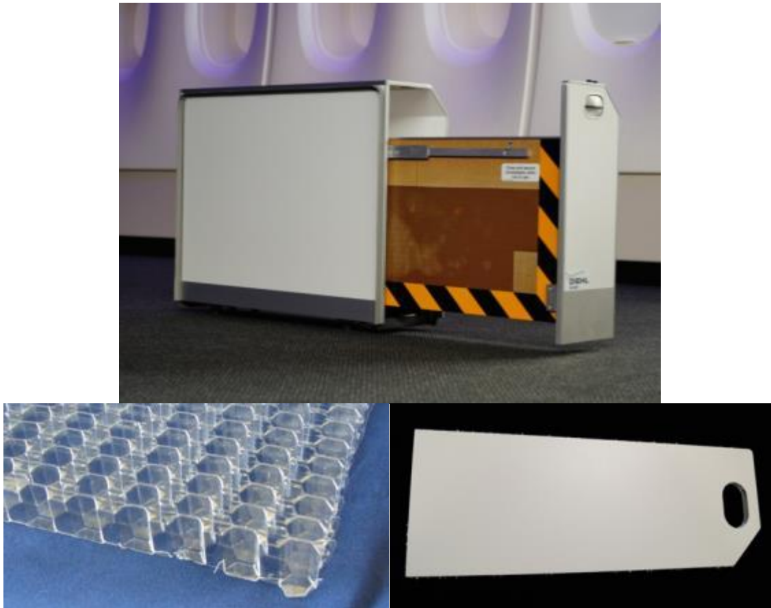
Figure 28. Stowage compartment of the Airbus A350 so called “Dog House” manufactured in INCOM project.
