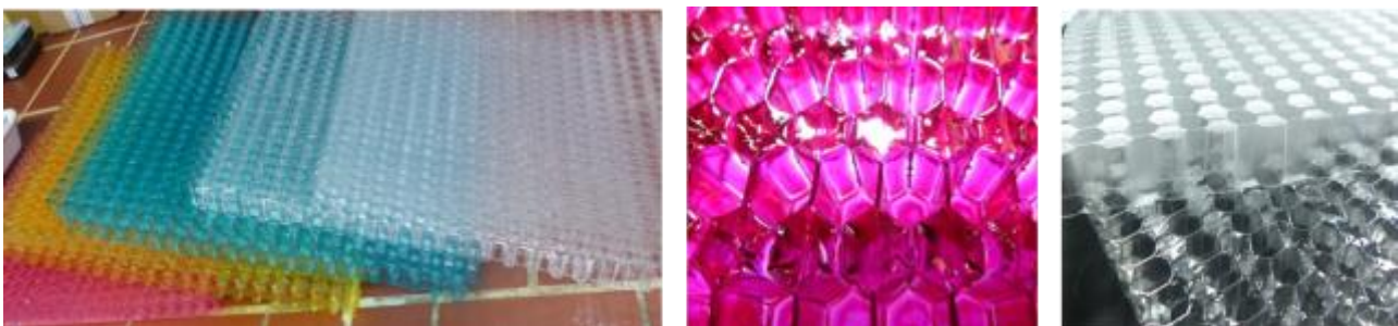
Figure 24. a) and b) UV curable non-filled colored coating. c) thermally curable coating with 10 % NFC. (Fh-ISC)
