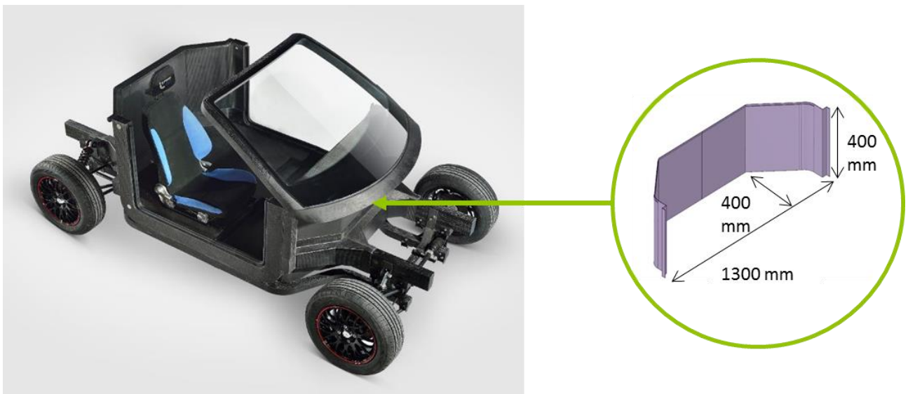
Figure 29. The front bulkhead of Axon Automotive Far Platform Chassis was selected as the demonstrator component.
