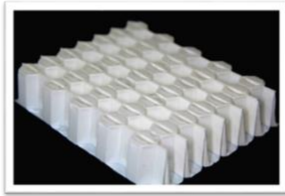
Figure 27. Sample of the 16mm fire-smoke-toxicity-qualified PC core.
