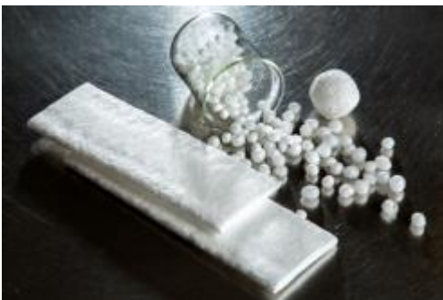
Figure 21. a) Extruded PLA foam and expanded PLA foam particle samples prepared at VTT. b) Small sandwich samples using extruded PLA foam and carbon fibre reinforced skins produced by CSI Composites.
