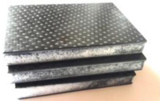
Figure 21. a) Extruded PLA foam and expanded PLA foam particle samples prepared at VTT. b) Small sandwich samples using extruded PLA foam and carbon fibre reinforced skins produced by CSI Composites.
