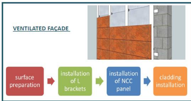
Figure 6 External Insulation walls – Ventilated facades
