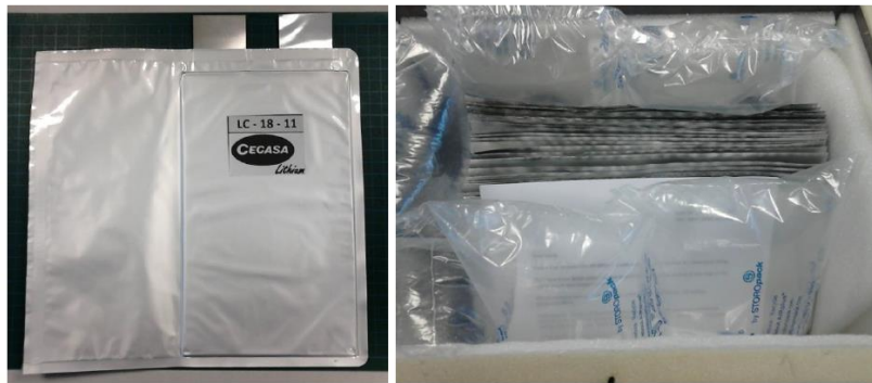
Figure 10. Sealed dry Gen#1 cells before supply to KIT for activation
