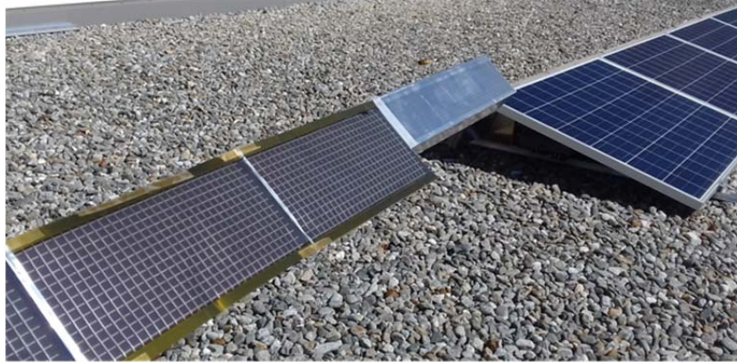
Figure 19: Task 7.2-proof of concept for SUN flexible PV solar panels (external benchmarking testing)
