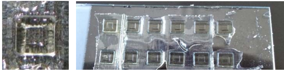
Figure 6: insulating material [TIGER IJ176-KK] printed simultaneously with support material [TIGER IJ176-KE]
