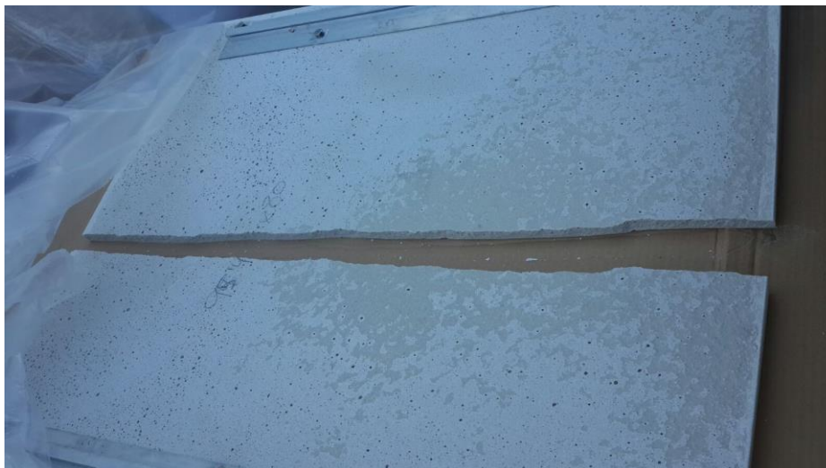
Figure 5.3: Broken panel after the first delivery.
