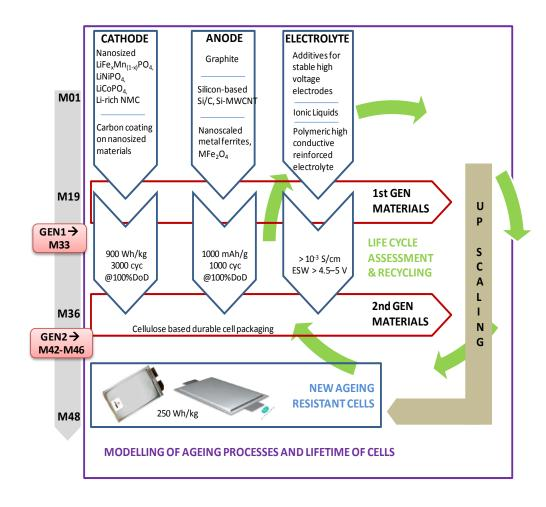
During the last year (M37-M48), efforts have been invested on the scaled-up manufacturing of electrodes (high-voltage cathode and optimized graphite anode) and
