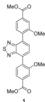
A new triaryl molecule based on functionalised bis(benzoic acid ester) and benzothiadiazole core has been applied as a single active layer in an OLED device. This very simple molecule emits intensively ( $> 5000 \text{ cd}\cdot\text{m}^{-2}$ ) from a combination of emissive states (exciton / electromer / exciplex / electroplex) to give white light with CIE coordinates of (0.38, 0.45) and a colour temperature of 4500K [2].
