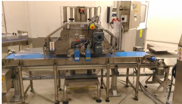
Inline SAFETYPACK Equipment for Tortilla Bread Products Inspection
