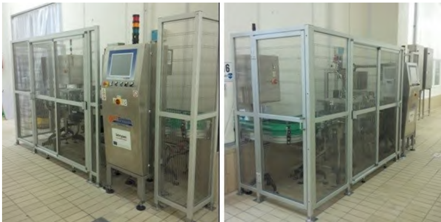
Inline SAFETYPACK Equipment for Mozzarella Products Inspection
