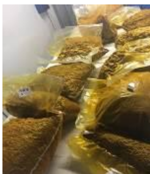
Fig. 10. Freeze-dried Westfalia-harvested biomass shipped in batches under vacuum for processing with scCO 2
