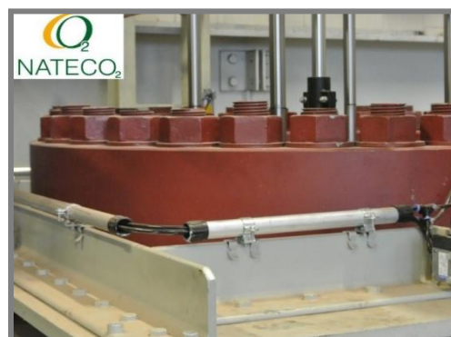
Fig. 11. Industrial plant HD12 for scCO 2 -extraction of algae biomass at
