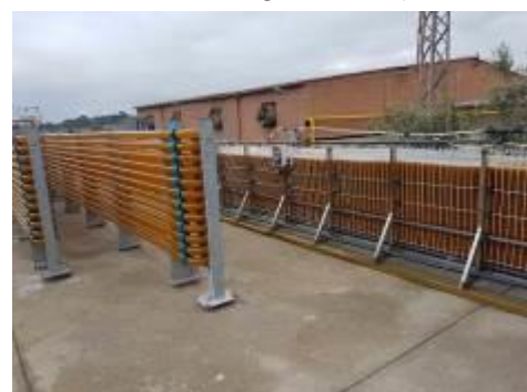
Fig. 7. A4F-Monzon closed flat-panel GW PBR (1,000L), & tubular PBR
