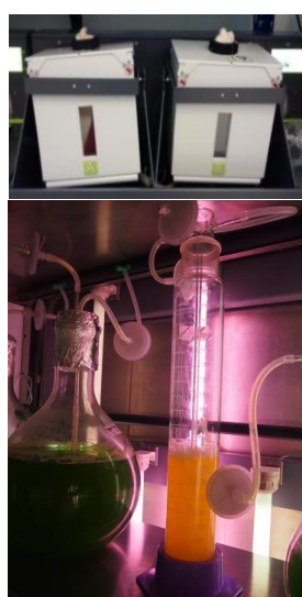
Fig. 3 Laboratory-scale PBRs for cultivating strains under strict control
