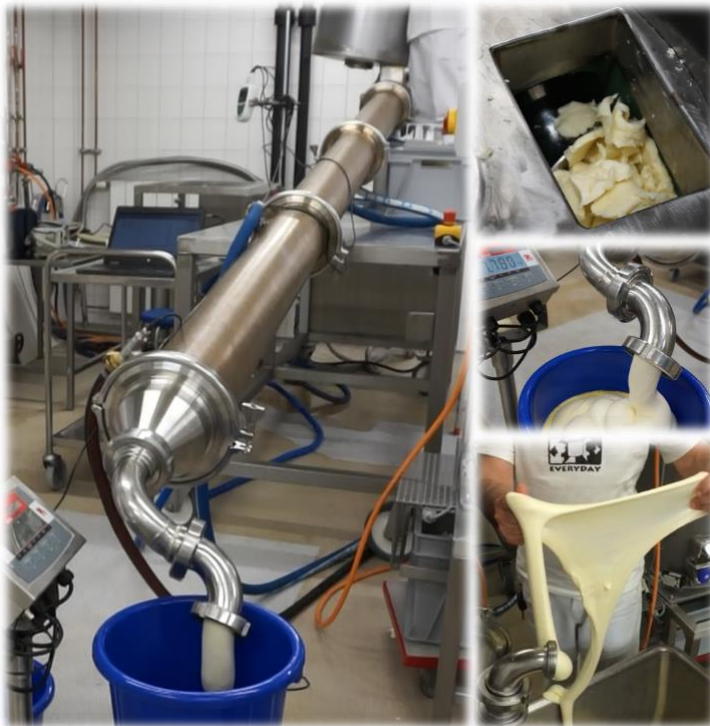
Figure 8: Large scale extrusion of cagliata in the facilities of the Dairy for Research and Training (University of Hohenheim); top: filling section, middle: extruded pasta-filata strand, bottom: stretching of pasta-filata.
