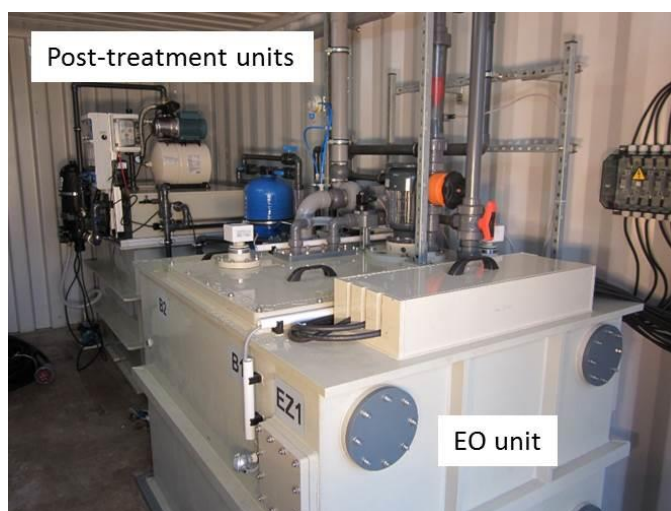
Figure 10: Electro-Oxidation Pilot Unit with post-treatment units
