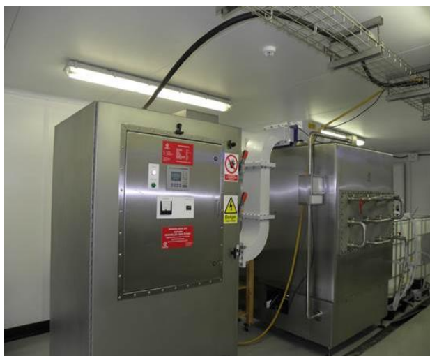
Figure 2: Microwave heating unit
