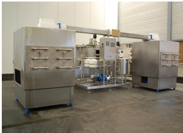
Figure 7: Microwave multipurpose unit (double reactor) for pre-heating, pasteurization and sterilization.
