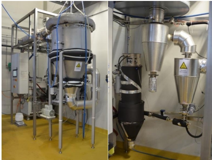
Figure 9: Super-heated-steam spray-dryer after several modifications during project
