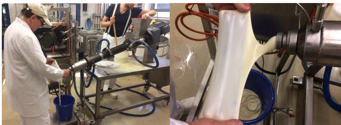
Figure 3: Production of Mozzarella using single-screw extruder at laboratory level
