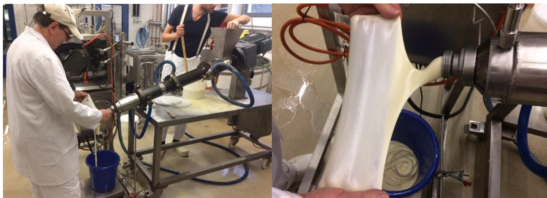
Picture 2: Production of Mozzarella using single-screw extruder at laboratory level
