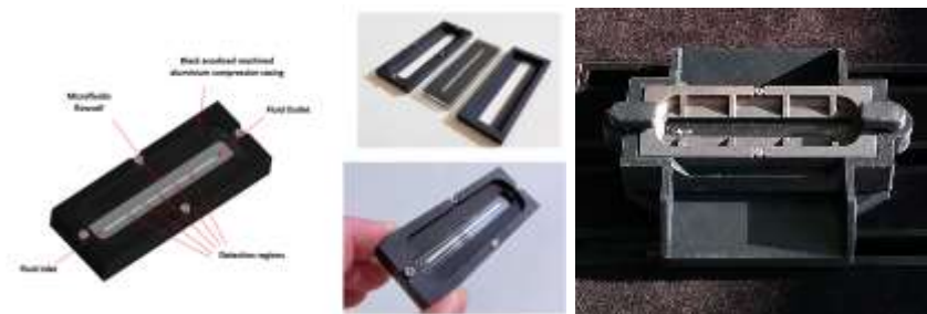
Fig. 3. Robust and simple to replace microfluidic flow cell.
