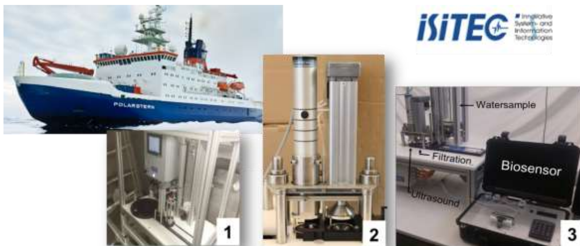
Fig. 1: Overview of the individual modules of the ADU: automated filtration unit for marine microbes (AutoFiM) installed on board RV Polarstern (1), sample preparation (2), and biosensor unit (3).
