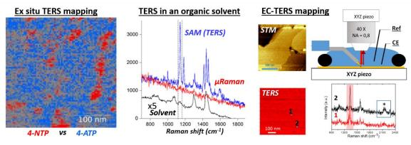
From left to right, ex situ STM-TERS mapping of 4-NTP/4ATP SAM mixture (300 x 300 nm<sup>2</sup>), TERS signature of a SAM covered by a layer of organic solvent, TERS imaging in water of a 4-NTP SAM on gold imaged using the EC-TERS cell, a partially insulated gold STM-TERS tip and an immersion objective. Similar developments for EC-AFM-TERS are under way.
