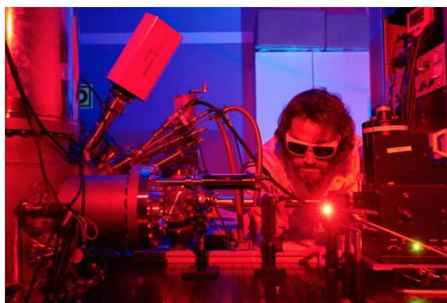
fellow combined a low temperature scanning tunnelling and force microscopies with a light excitation and detection set-up, to resolve at the atomic scale both electronic structure and light scattering/emission by the atomic-sized antennas in response to optical/electron excitations. Specifically, he constructed an optical table coupled to our low-temperature STM via a set of mirrors and lenses. The system has been tested successfully by detection of plasmonic light emitted from a gold tip.
