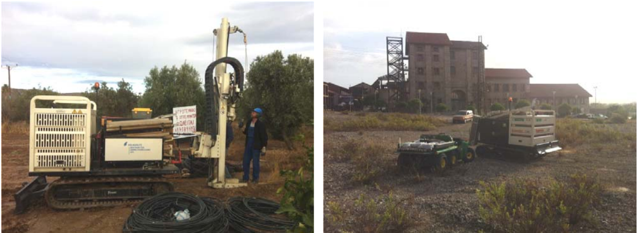
Fig. 2: Direct push activities for the characterization of the subsurface in the Lavrio catchment (left) and for the selection of the optimal location for the infiltration basin at the Lavrio Technological and Cultural Park (right).
