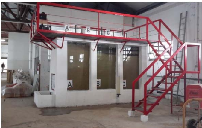
Fig. 21: Sandbox model to study infiltration under well-defined conditions to get high quality data (left), and schematics of the model with dimensions (right).
