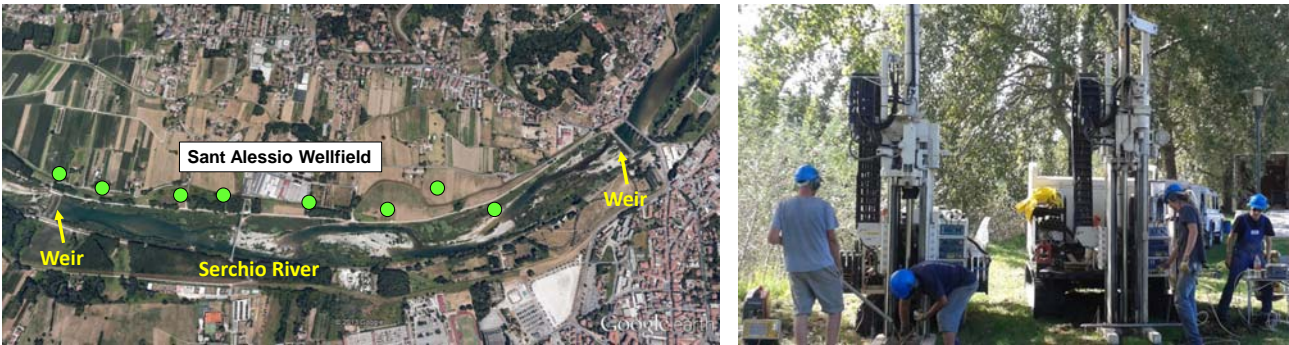
Fig. 12: Sant'Alessio well field at the Serchio River in Lucca, Tuscany (left), and Geoprobe activities for subsurface characterization of the aquifer (right).
