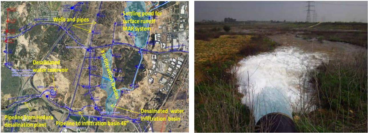
Fig. 14: Location of the infiltration ponds of the Menashe field site with the infiltration pond for desalinated water (left), and filling of the pond with desalinated seawater for infiltration (right).
