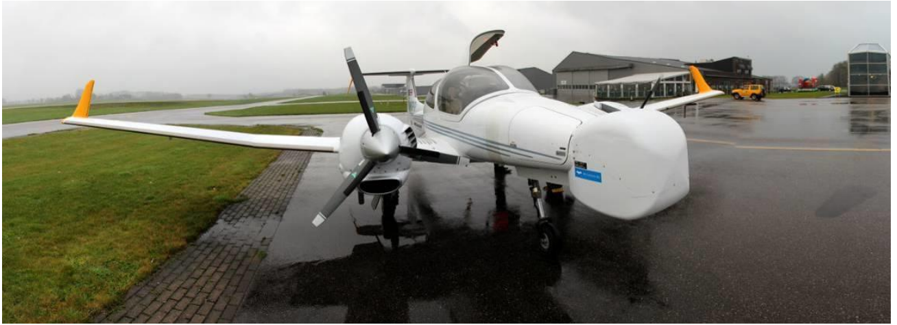
Nose pod-equipped DA42 at the airport of Teuge (NL) during the first XWALD measurement campaign.
