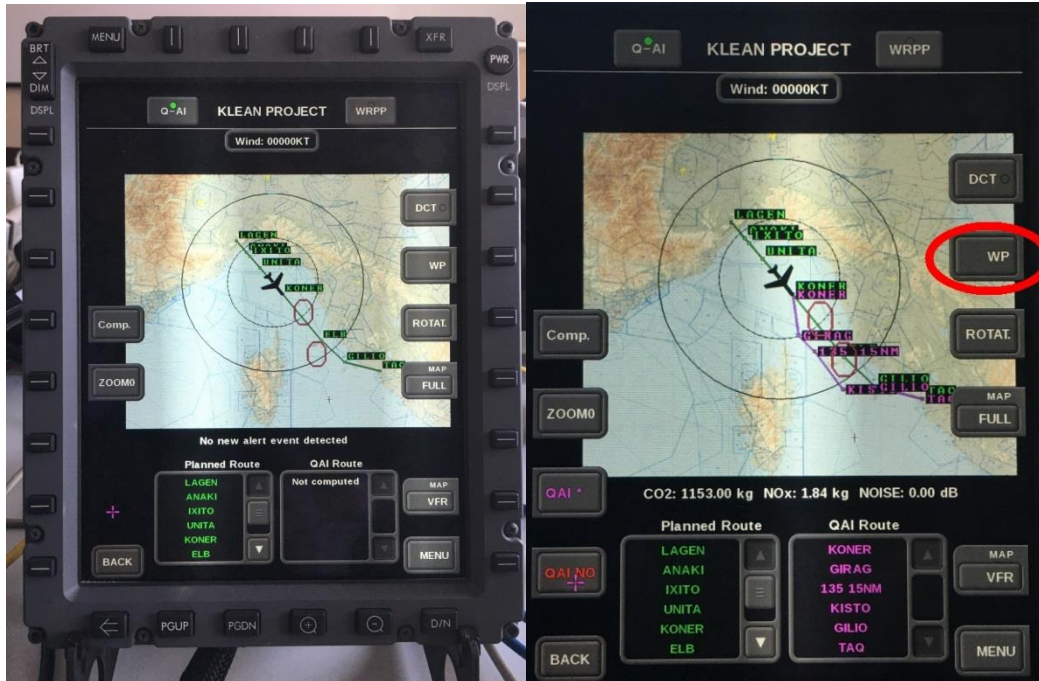
The EFB GUI main screen soon after the no flight zone event (left), and after (right) presentation of routes and waypoints (planned route and its waypoints are all in green, the Q-AI proposed route and its waypoints are in magenta. The WP button switches on/off the visibility of labels.
