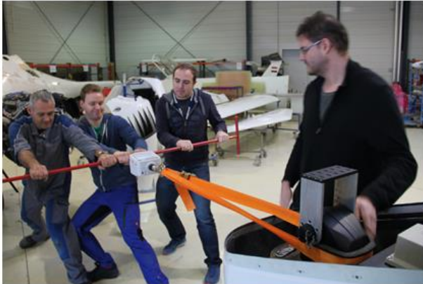
Radar installation and certification on the DA-42 at Diamond facilities, in Austria. From top left, clockwise: CAD study of potential location for different radar subsystems; actual implementation in the front nose; avionics instrumentation monitored during RFI tests for certification; mechanical check of installation for certification.
