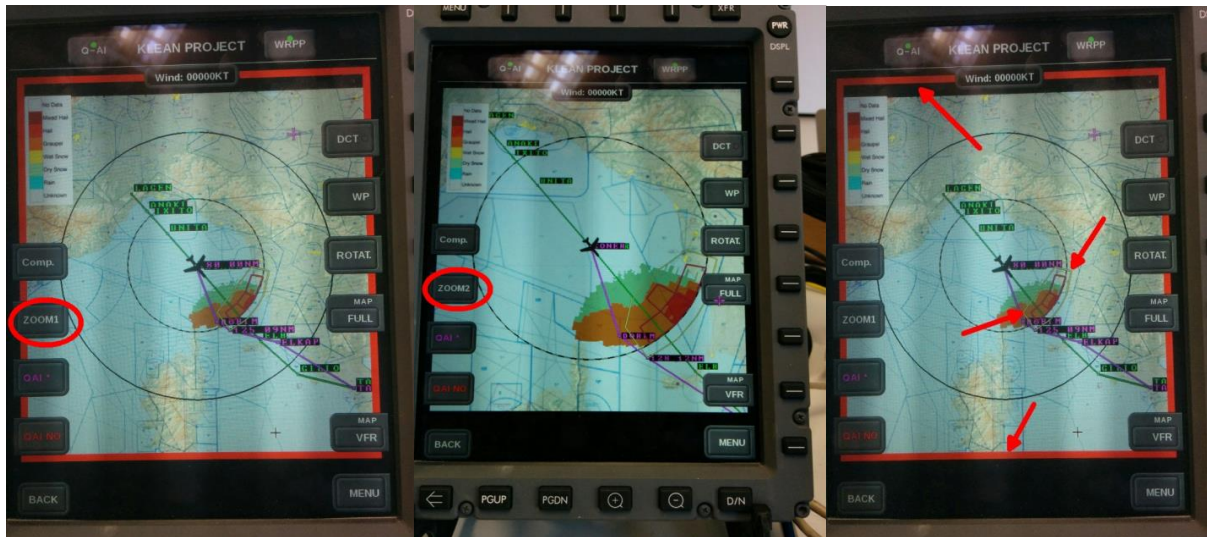
EFB screen - Comparison of zoom level 1 (left) and level 2 (center). Circles are at 40 and nm. Red arrows (left) indicates the 1 Hz red lines blinking corresponding to risk area
