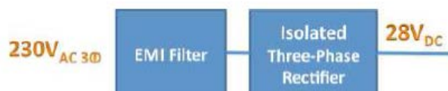
Isolated Three-Phase Rectifier.
