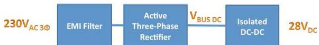
Electrical architecture for high performance TRUs.
