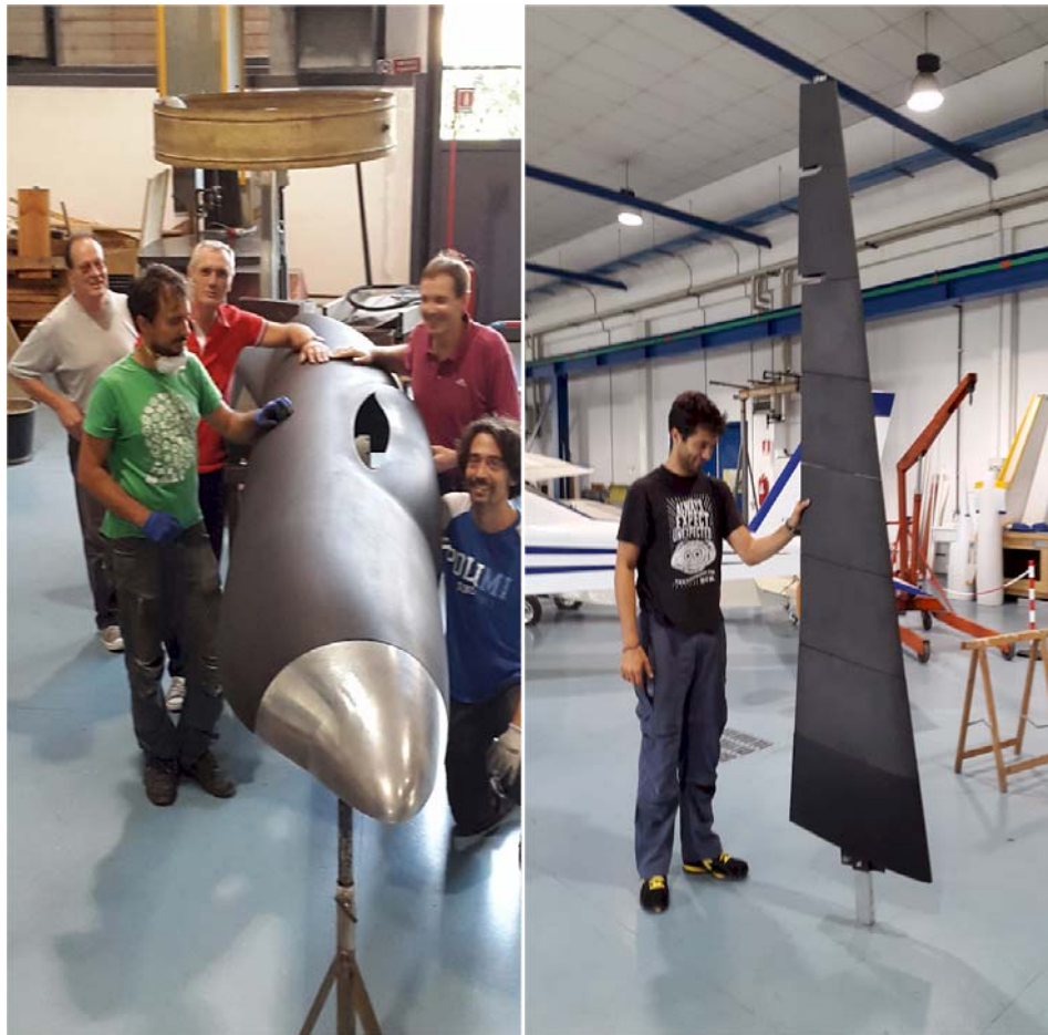
Figure 3: Fuselage and wing during the final assembling.
