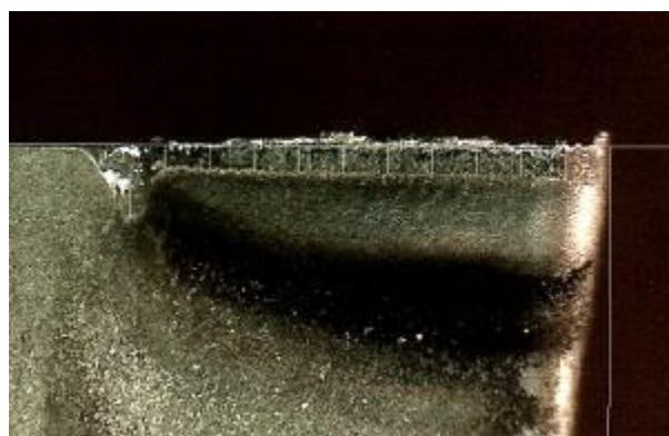
Figure 15. Flank wear tool.
