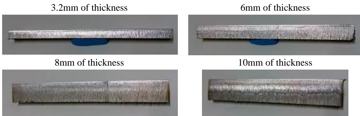
Figure 36. LB cuts in different thicknesses of Alloy 718
