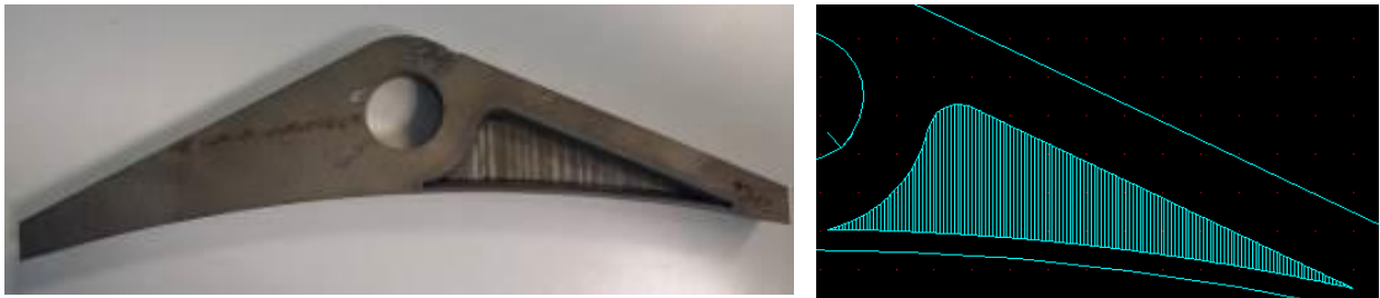
Figure 4. AWJ demonstrator over Alloy 718.
