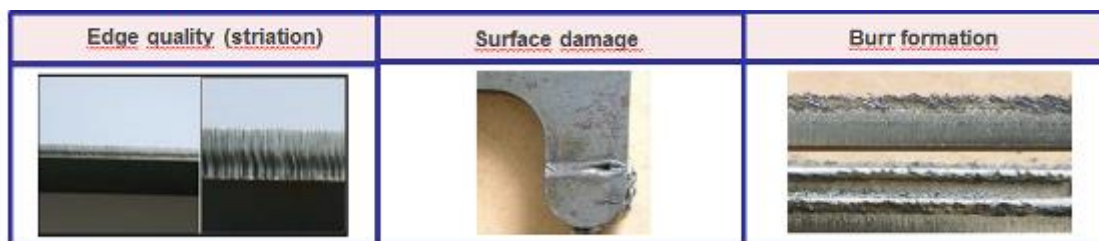
Figure 31. Defects produced by LB cutting
