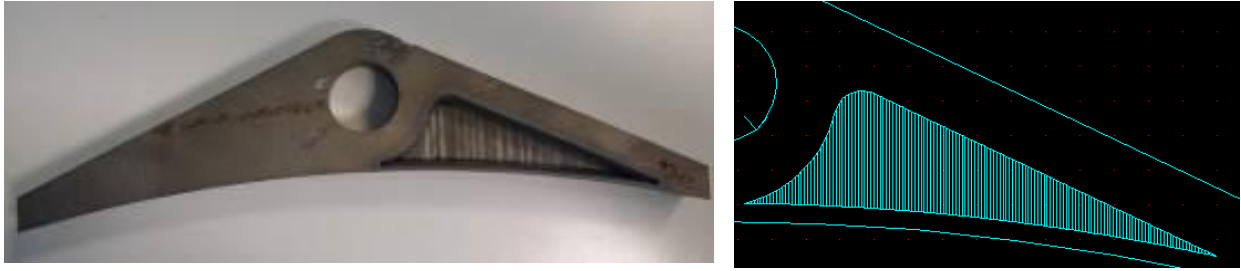
Figure 4. AWJ demonstrator over Alloy 718.
