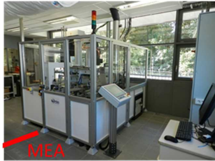
Figure 4: available automated MEA assembling machine (CEA)
