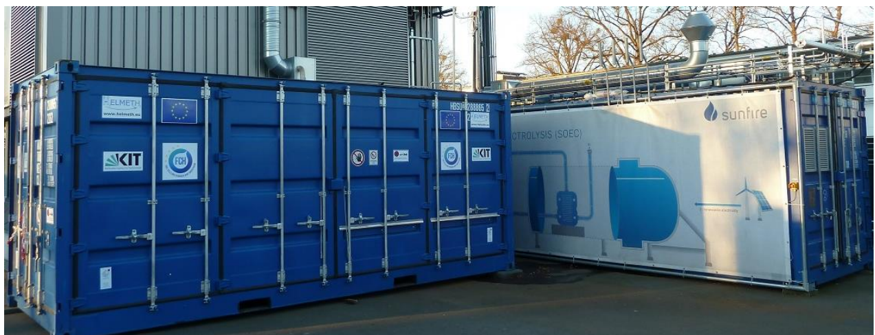
Figure 2: Final HELMETH prototype, consisting of the methanation module (left container) coupled to electrolyser module (right container)
