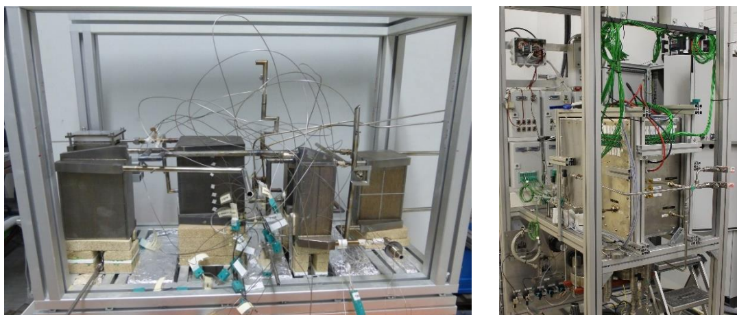
Figure 8: Fuel processor during installation of reactors and thermocouples at Fraunhofer IMM (left), and fuel processor installed to test bench at VTT (right).
