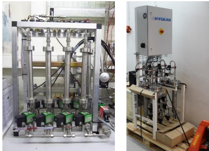
Figure 9: Lab scale PSA unit at UPorto (left) and prototype PSA unit by HyGear (right).
