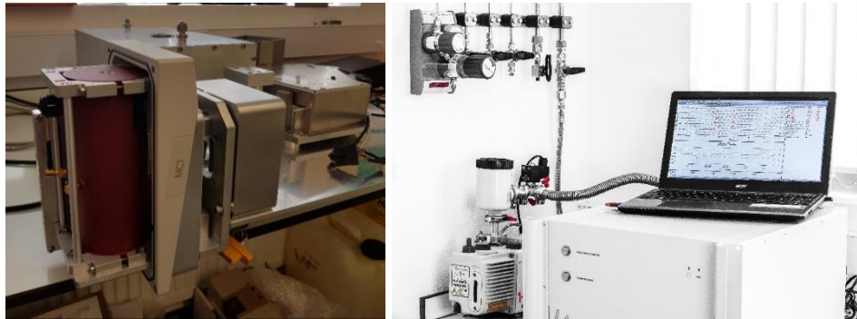
Figure 4. Left: HyCoRA FTIR assembly showing Liquid Nitrogen cooled detector assembly that can be inter-changed with DTGS for fieldwork. Right: Mass Spectrometer analyser built for HyCoRA project
