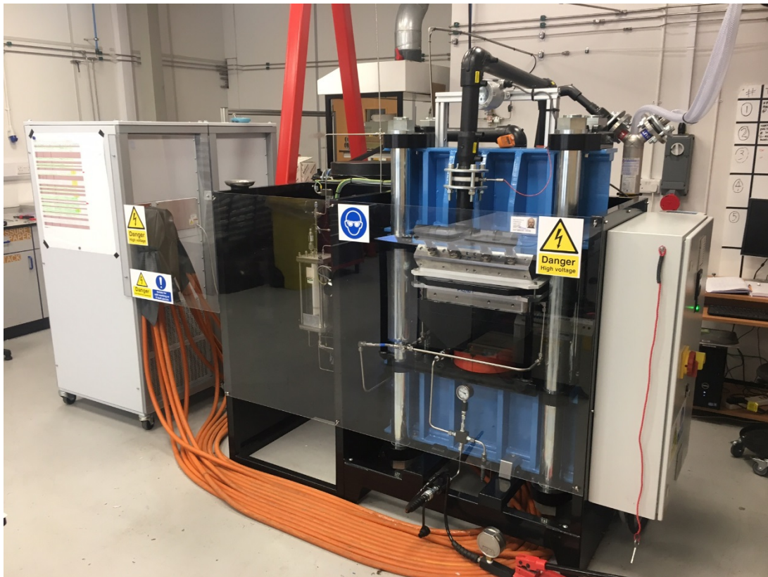
Figure 21: Finalised balance of plant, skid and short stack during testing.
