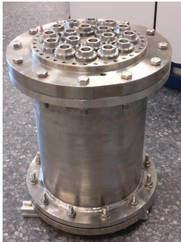
Figure 4. Multi-tubular 1 kW 20 bar electrolyser module unit for 18 tubes with easy tube insertion from cold side and individual monitoring, shut-off, and replacement during operation.
