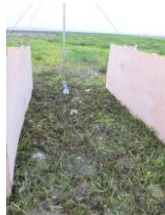
Fig 3 A) The winter field flume experiment at the Tillingham marsh to measure sediment deposition/canopy morphology interactions. OBS = Suspended sediment profilers (ASM-IV), ADV = Flow velocimeter. B) and C) the plant canopy before and after final manipulation during the summer field flume experiment.
