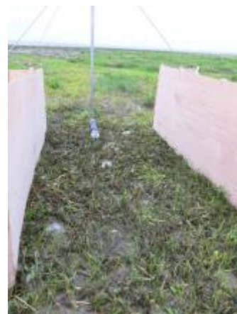
Fig 3 A) The winter field flume experiment at the Tillingham marsh to measure sediment deposition/canopy morphology interactions. OBS = Suspended sediment profilers (ASM-IV), ADV = Flow velocimeter. B) and C) the plant canopy before and after final manipulation during the summer field flume experiment.
