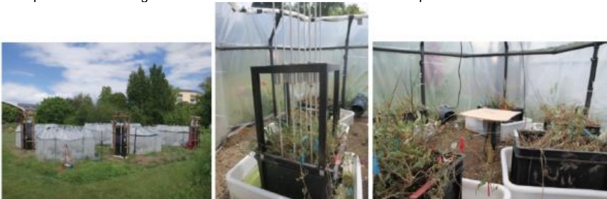
Figure 1) The mesocosm experiment constructed at the Cambridge University Botanic Gardens where saltmarsh blocks were grown under different climate change scenarios to measure the effects of elevated CO 2 and eutrophication on surface elevation change (Reef et al. 2016).
